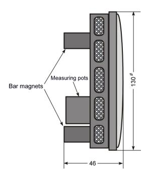
The thermo-hygrometer contains a precision humidity meter and two bimetal measuring systems. Here the temperature, the relative humidity, the saturation moisture and the dewpoint can be read off directly following the curves from the point of intersection of the surface temperature pointer and the relative surface humidity pointer. The back of the case is fitted with 3 strong bar magnets for steel part usage.
